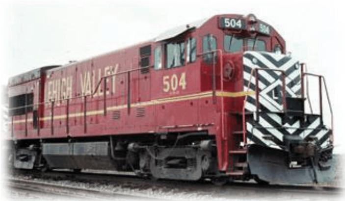
The locomotive is one of 12 GE, model U-23B, diesel electric locomotives built in 1974 for the Lehigh Valley Railroad. Upon inclusion into Conrail in 1976, the “U-Boats”, as they were fondly known, were painted blue, renumbered, and reassigned to various portions of Conrail’s far-flung system. Upon retirement from Conrail, many were scrapped, and the remaining few were sold to private companies in need
